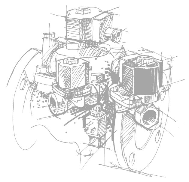
Solenoid valves 2/2-way assisted lift operated Type EV250B
